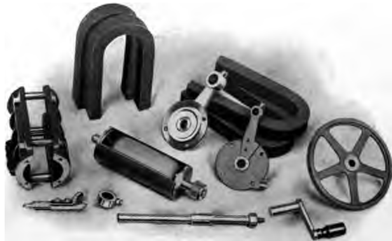
FIG. 5.—MAGNETO GENERATOR DISSECTED.
